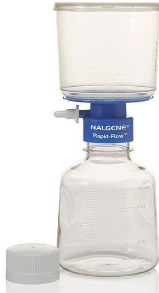
Filtration normally with a 0.2µm filter
