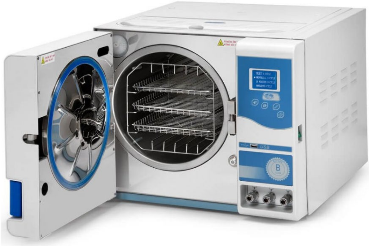
Autoclave Heating to 121-132°C
